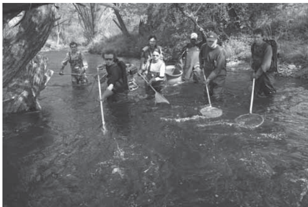
Electrofishing using backpack electrofishing equipment
