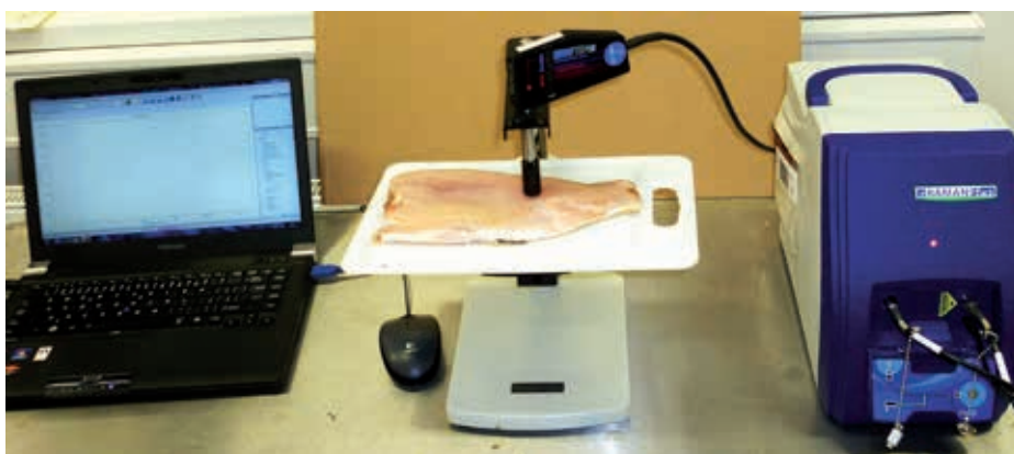
Raman spectrometer for non-destructive analysis of fish flesh quality.
