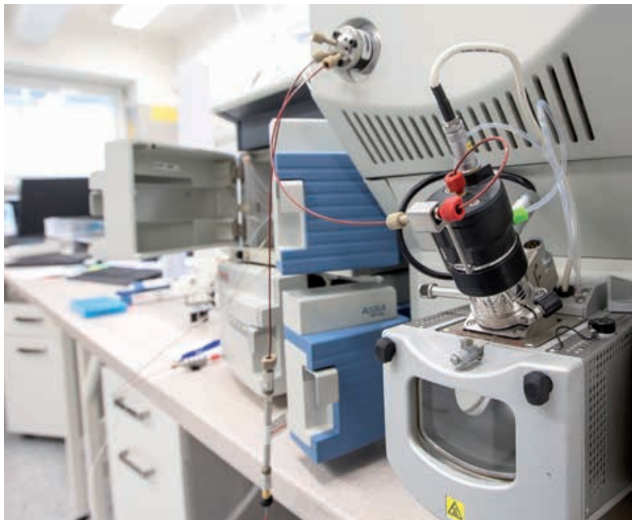
Two-dimensional liquid chromatograph in the Laboratory of Environmental Chemistry and Biochemistry.
