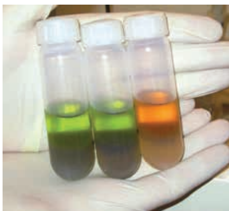
Extraction of lipids from pond plankton samples (left) and fatty acid methyl esters (FAME) in vials ready to gas chromatography (GC) analysis.
