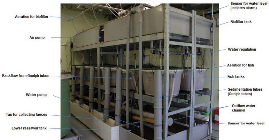
Fig. 2. Snapshot of our in-house Guelph system used for digestibility trials. (Photo: laboratory archive).
