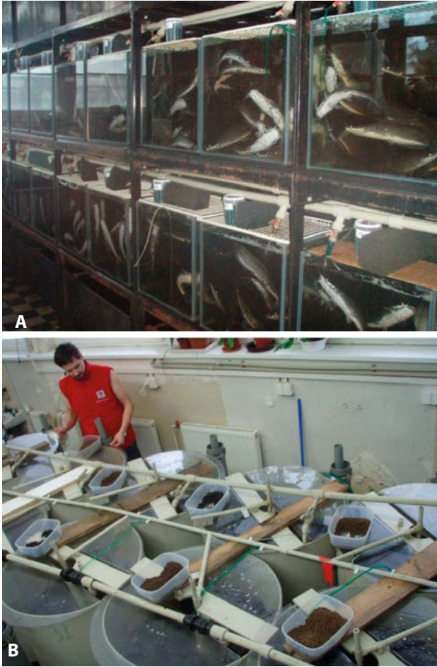
Fig. 28. Interior of aquarium room of the Institute of Aquaculture FFPW USB in České Budějovice: experimental aquariums (A) and circular tanks (B) in recirculating aquaculture systems with course of feeding tests in African sharptooth catfish. Photo by J. Kouřil
