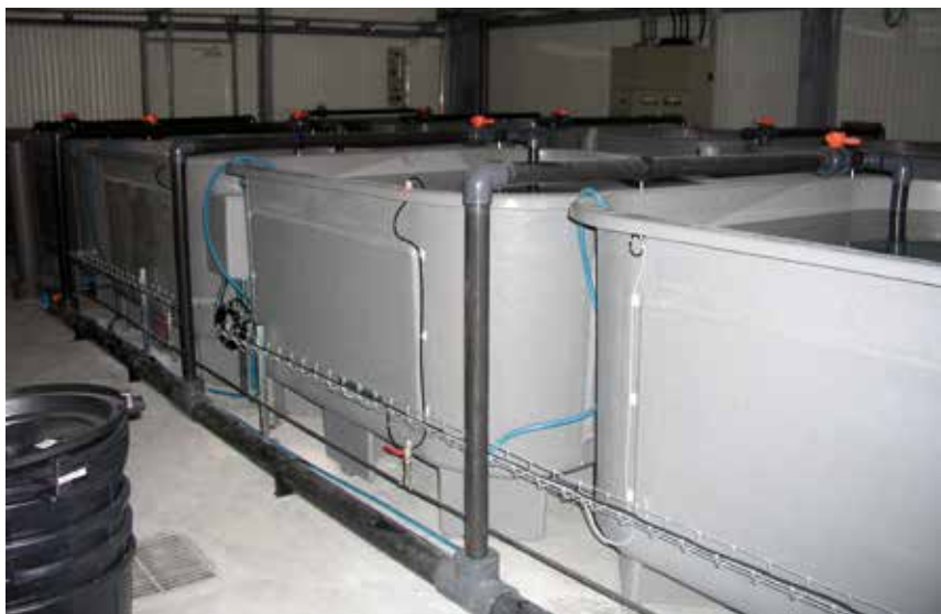
Fig. 4. Suitable recirculating aquaculture system used for intensive culture of older pikeperch, Sander lucioperca (L.) in Asialor Ltd. company, France (photo T. Policar).
