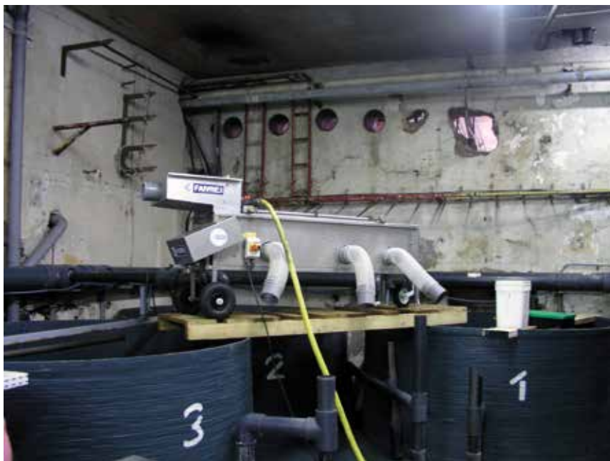
Fig. 16. Automatic sorter used in commercial intensive farms of Eurasian perch, Perca fluviatilis (L.) and pikeperch, Sander lucioperca (L.) in Lucas Perch Ltd. company, France (photo T. Policar)
